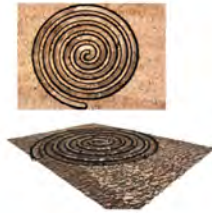
Spiral Channel (100 micron) Microfluidic Application
